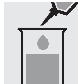
Add 0.20 ml perchloric acid 70–72 % GR with pipette and mix.
